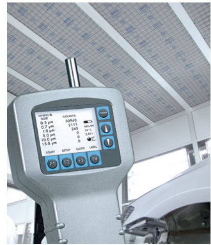
Raster measurement of sink rates in the spray booth
