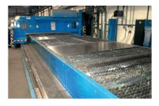
Laser cutting plant for the extraction of steel and aluminum dust, which need to be removed during the cutting of ship components.
