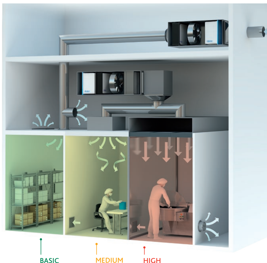
Illustration of a typical multi-stage air handling system supplying clean air to a food production plant
