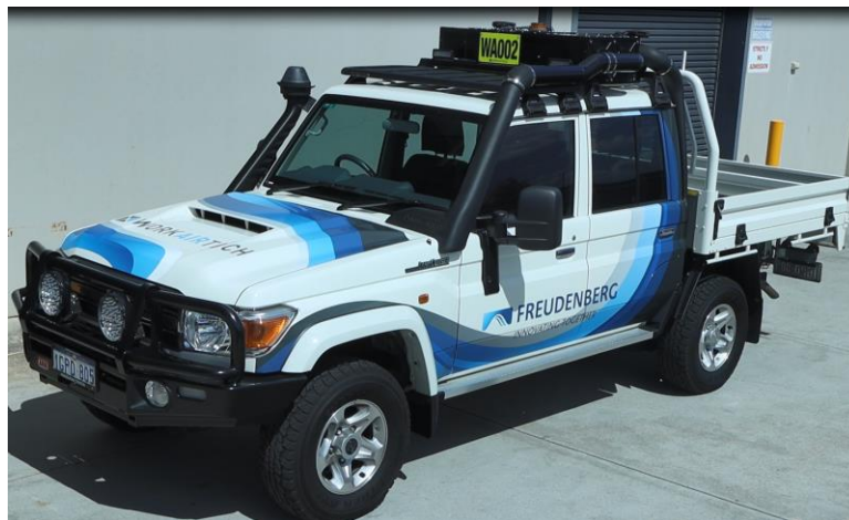
Figure 1: Toyota Landcruiser with Freudenberg S.A.F.E air cabin protection system
