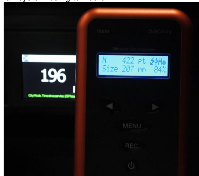
Figure 3: Discmini reading 420 particles per cubic centimetre and pressure reading +196 Pa (doors closed)
