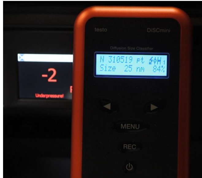
Figure 2: Discmini reading 310K particles per cubic centimetre and pressure reading -2 Pa (doors open)
